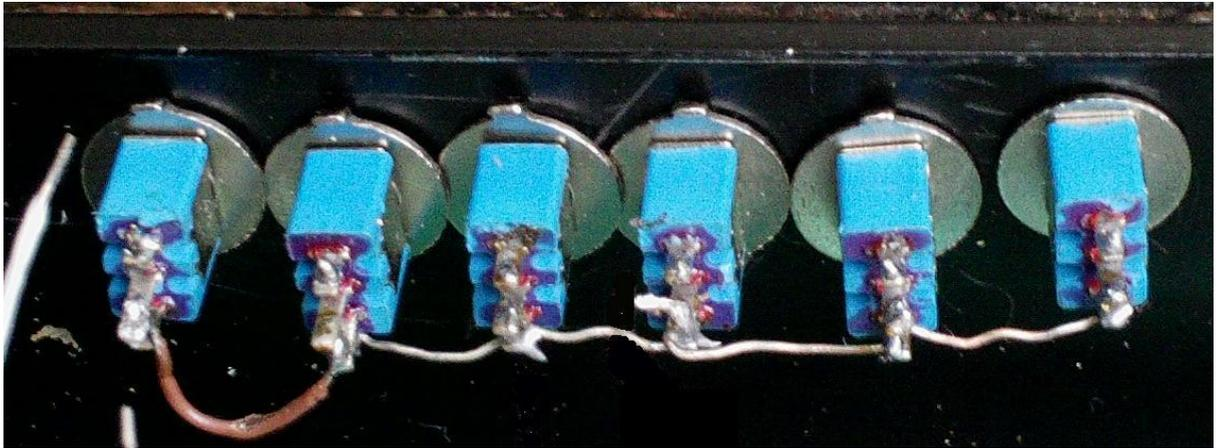
5. Cut holes to mount 6 additional large jack sockets on the rear panel. Label the first as 'Mix'. Label the others from 1 – 6.
